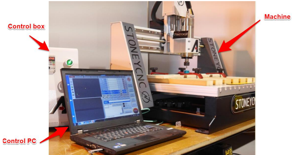
Figure 18: Locate control PC near to machine and control box
