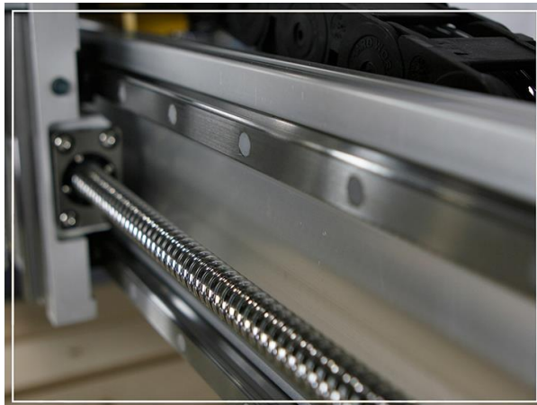
Figure 68: Weekly (best case daily) cleaning and application of light oil externally to screws and rails with cloth and light oil.
