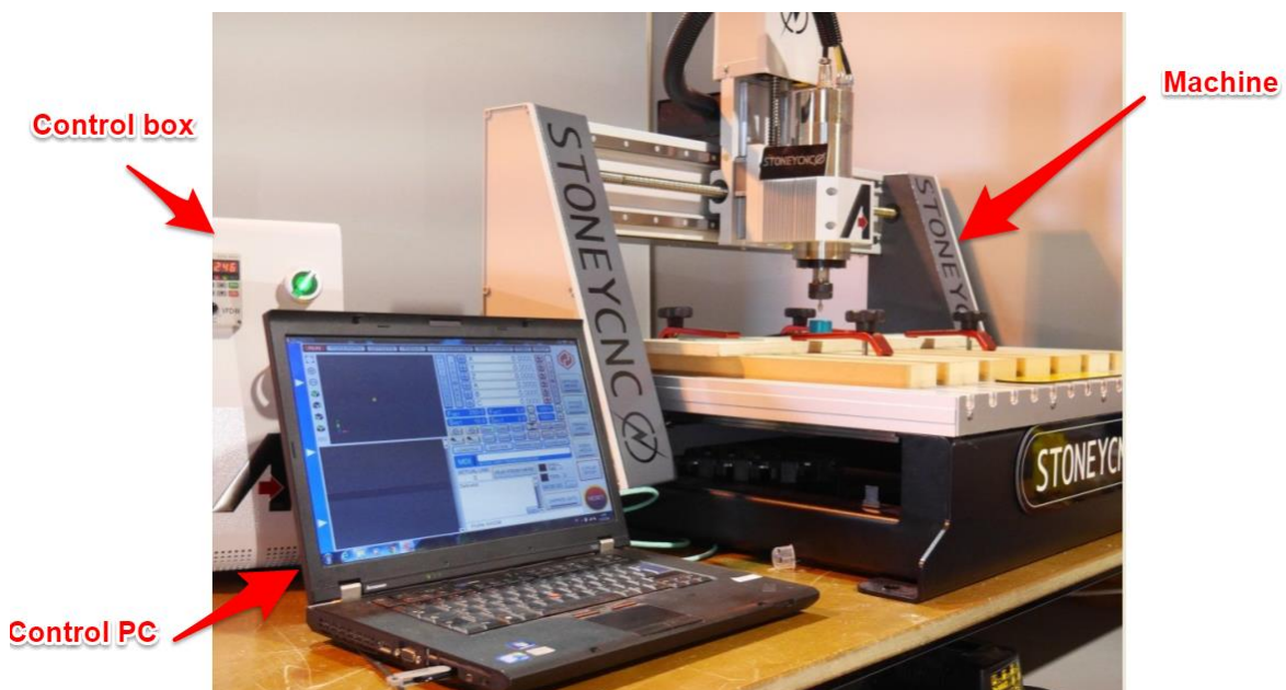
Figure 24: I2R AR series router sitting next to controller and PC
